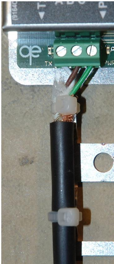
The simplest way to accomplish this is to remove the outer insulation of the cable and to fold down the screen on the outside of the insulation and to secure the cable with the straps supplied.
