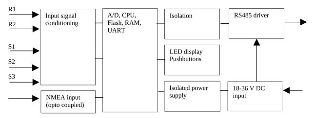
The power supply for the internal circuitry is isolated from the ship's power supply input, and the NMEA input for set-up/alignment (where needed) is opto-isolated.
