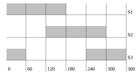
The similarity of the synchro format should be noted, although the three phase signals can only assume one of two different states, on and off, meaning that each revolution is only subdivided into six sectors, each  $60^{\circ}$ .
